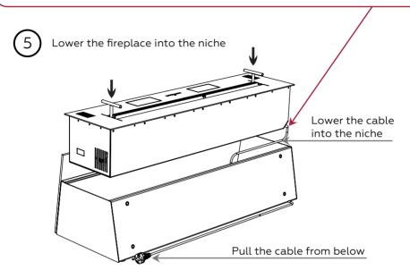
Unscrew the mounting handles after installation
